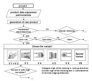
Figure 6: Part of an Algorithm for Generation of Raw Products for a Seiatsu Molding Maschine
